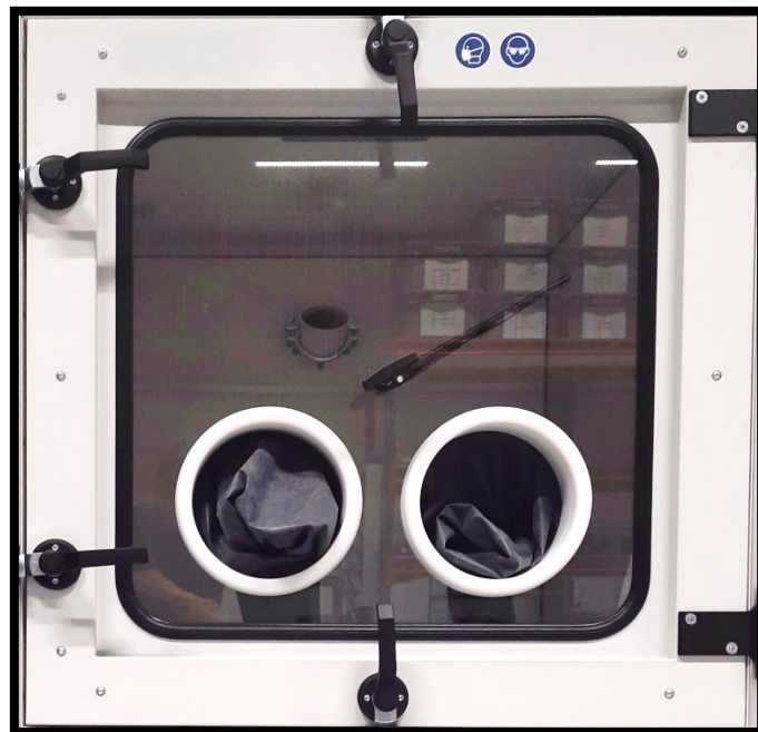
Pair of gloves installed in the door
