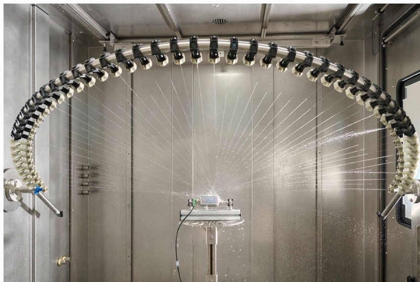
R800 swivel tube in an SPKR800
