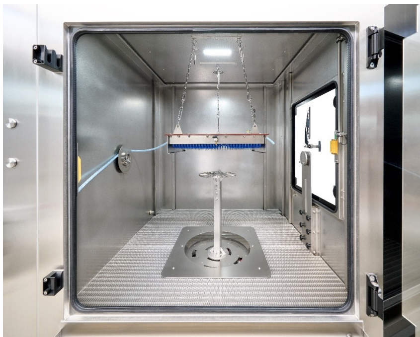
Dripping water box TG 64 in SPK R600
