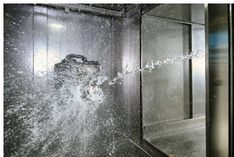
UL 50 Hose Down test
