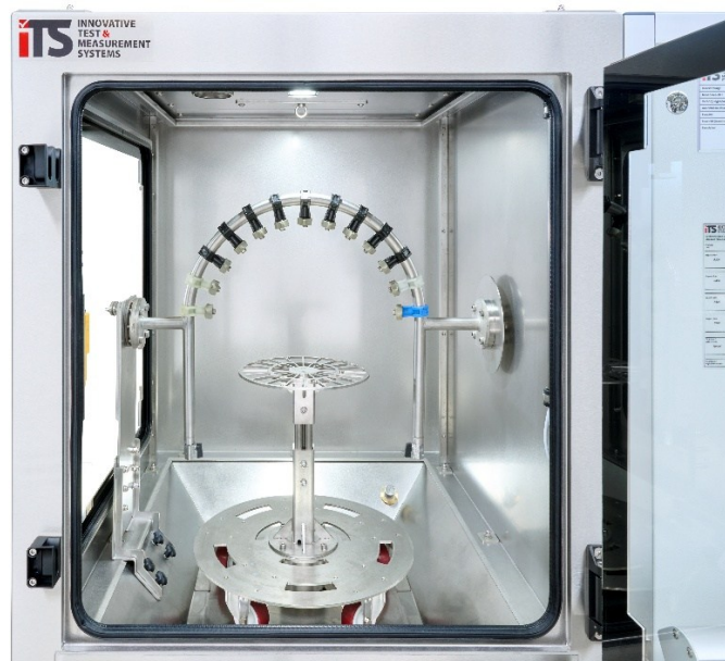
Interior view: R200 swivel tube in a SPK R200.
