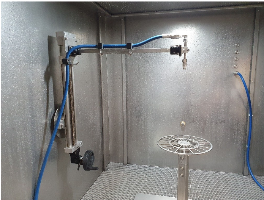
Swivelling lance for IPX9K
