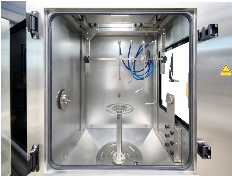
IPX9K high-pressure lances in an SPK R400
